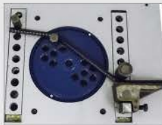
LEFT/RIGHT STANDARD Produce Double Bends and bend from Left to Right
